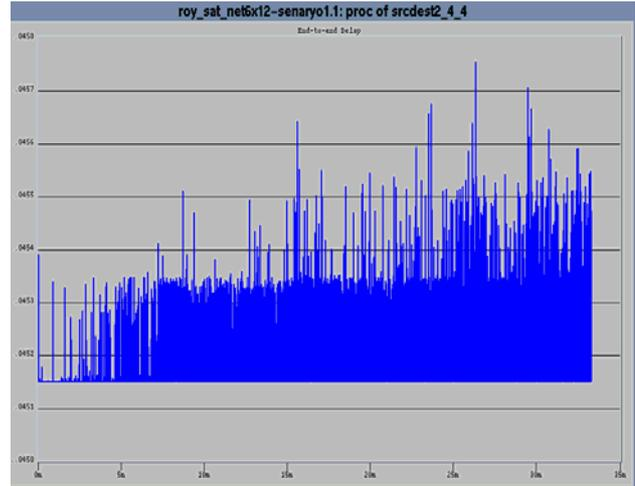
Figure 11. End-to-end delay plot of traffic from (1,2) to (2,4).
