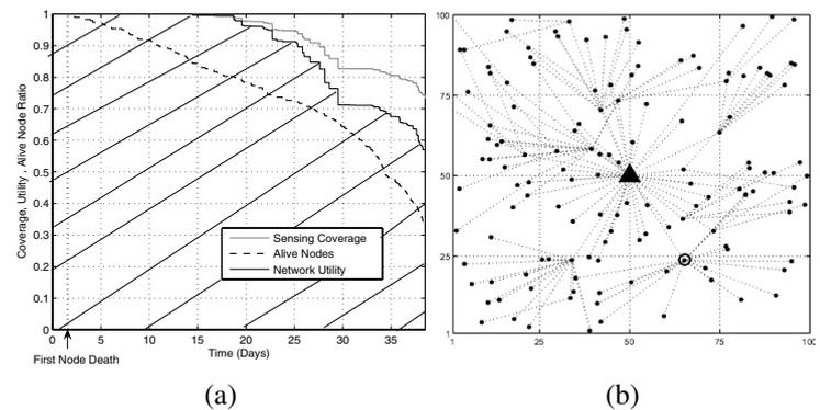
Figure 5: (a) Evolution of the network parameters (300 Nodes, BPR case) (b) Static routing paths of MER. Circled node denotes the first node to die
