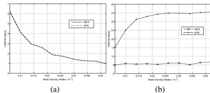
Figure 6: Performance comparison of the routing algorithms MER and BPR (a) Lifetime metric is FND (b) Lifetime metric is WCOT
